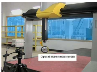
Fig. 3 Device for camera parameters calibration
