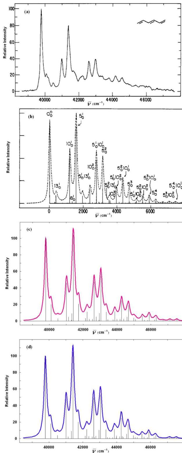
Figure 1. The  $1^1A_g \rightarrow 1^1B_u$  absorption spectrum of hexatriene. (a) experimental spectrum in jet-cooled from ref. 12, (b) calculated spectrum using PPP/CI theory from ref. 16, (c) calculated spectrum using displaced-distorted model, and (d) calculated spectrum using displaced-distorted-rotated model
