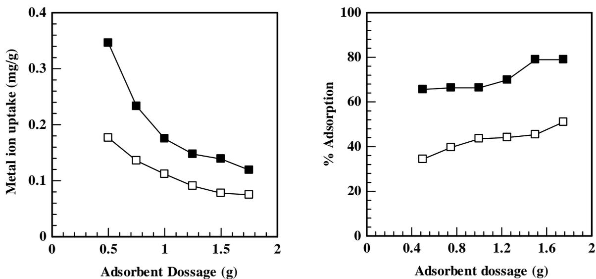
Fig. 7. Effects of adsorbent dosage and % adsorption on Pb(II) (■) and Cd(II) (□) biosorption; metal ions solution volume 25 mL; concentration of solution 10 mg/L; pH of solution 4; adsorbent weight 0,5 g; contact time 15 min; agitation speed 100 rpm for Pb(II) and 150 rpm for Cd(II); ratio alginat : biomass 1:0,5 for Pb(II) and 1:1 for Cd(II)
