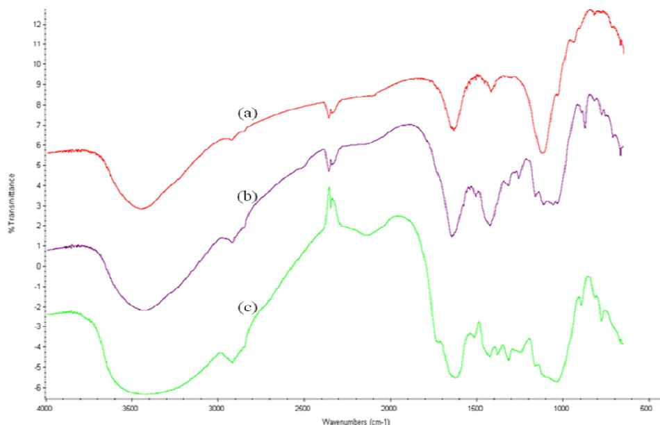
Fig. 2. FTIR spectra of *Arenga pinnata* shell beads sodium alginat (a), before (a) and after (b) adsorption
