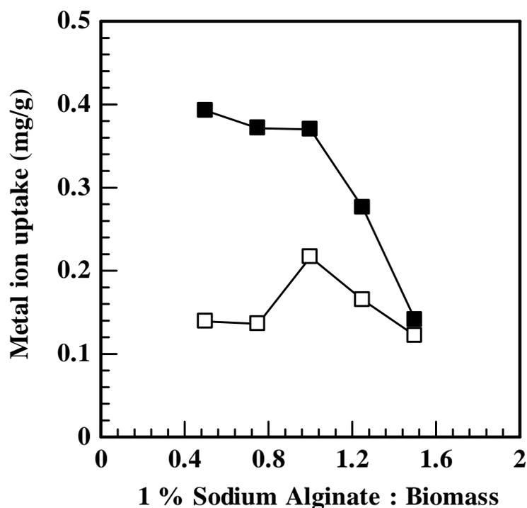
Fig. 6. Effects of ratio alginate : biomass on Pb(II) (■) and Cd(II) (□) biosorption; metal ions solution volume 25 mL; concentration of solution 10 mg/L; pH of solution 4; adsorbent weight 0,5 g; contact time 15 min; agitation speed 100 rpm for Pb(II) and 150 rpm for Cd(II)
