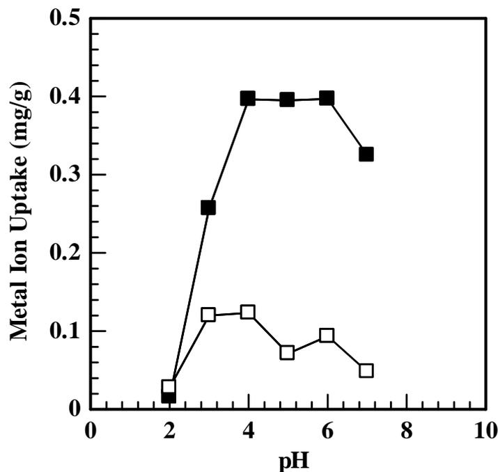
Fig. 3. Effects of initial pH on Pb(II) (■) and Cd(II) (□) biosorption; metal ions solution volume 25 mL; concentration of solution 10 mg/L; adsorbent weight 0,5 g; contact time 60 min; agitation speed 100 rpm
