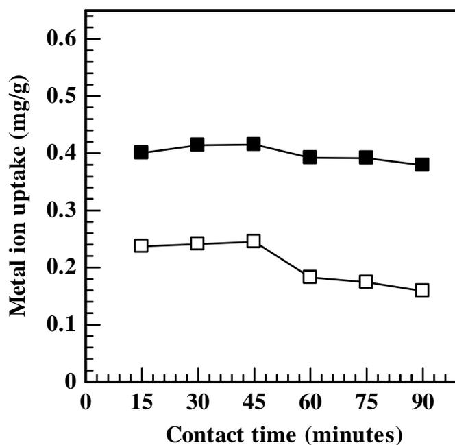
Fig. 4. Effects of contact time on Pb(II) (■) and Cd(II) (□) biosorption; metal ions solution volume 25 mL; concentration of solution 10 mg/L; pH of solution 4; adsorbent weight 0,5 g; agitation speed 100 rpm
