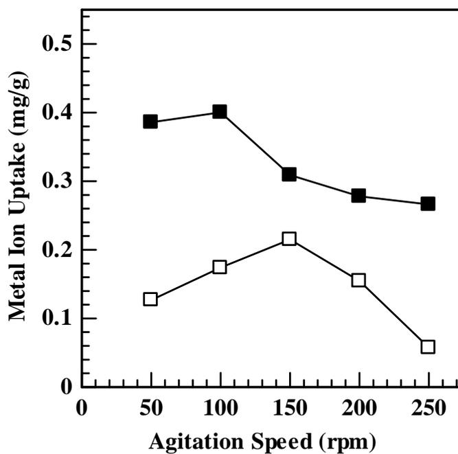
Fig. 5. Effects of agitation speed on Pb(II) (■) and Cd(II) (□) biosorption; metal ions solution volume 25 mL; concentration of solution 10 mg/L; pH of solution 4; adsorbent weight 0,5 g; contact time 15 min
