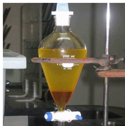
Fig: 3 Separation of two phases are carried out
