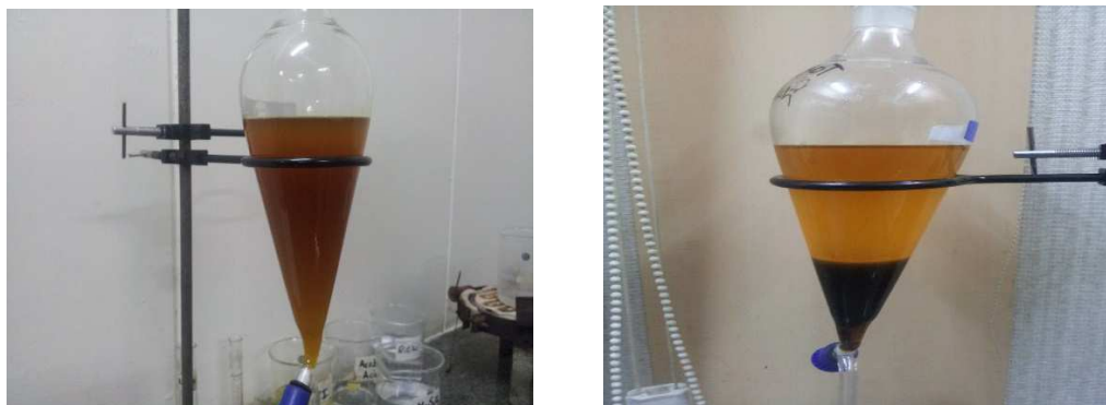
Fig: 3 Glycerine and waste cooking oil methyl ester mixture, before and after separation
