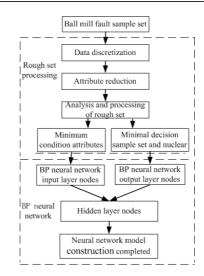
Fig. 1. The flow chart of ball mill fault diagnosis
