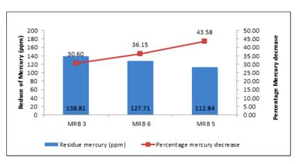
Figure 1: Residu mercury and percentage mercury decrease on day thirty after incubation using superior mercury resistant bacteria isolate *ex-situ* with simple open bioreactor
