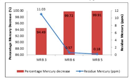
Figure 4: Residu mercury and percentage mercury decrease on day sixty (two months) after incubation using superior mercury resistant bacteria isolate ex-situ with simple closed bioreactor
