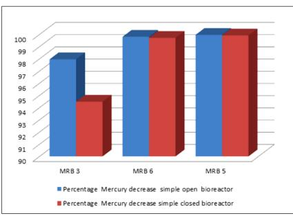
Figure 5: The comparison of superior mercury resistant bacteria using simple open and closed bioreactor on the mercury decrease percentage on day sixty (two months) after incubation
