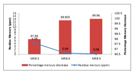
Figure 2: Residu mercury and percentage mercury decrease on day sixty (two months) after incubation using superior mercury resistant bacteria isolate *ex-situ* with simple open bioreactor
