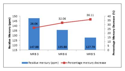
Figure 3: Residu mercury and percentage mercury decrease on day thirty after incubation using superior mercury resistant bacteria isolate *ex-situ* with simple closed bioreactor
