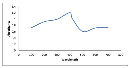
Figure 5. UV-Vis absorption spectra of silver nanoparticles biosynthesized from Calothrix marchica
