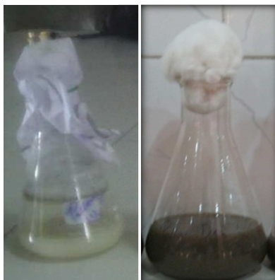
Figure 1: Color change to reddish brown after treating filtrate of endophytic Aspergillus sp. , with 1mM AgNO 3 .nanoparticles in the reaction mixture
