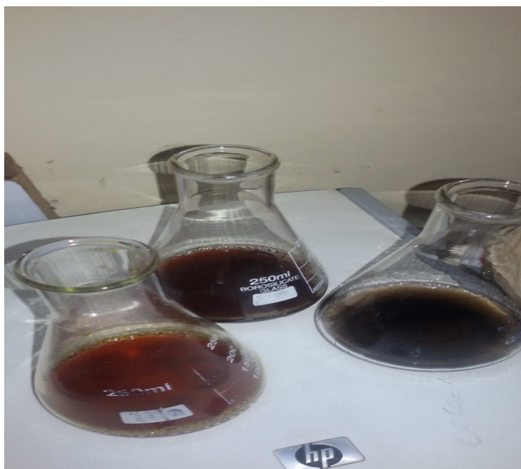
Figure 1 (a): Hydro-alcoholic solvent extraction of mushroom samples
