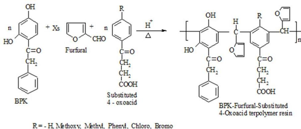
Scheme 1. Synthesis of terpolymer resin
