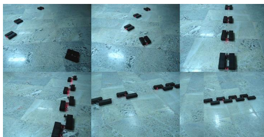
Fig. 12. Process of aggregation and docking among multi-robots
