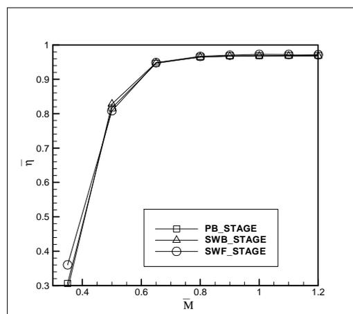
Figure 4. Variable flow stage average isentropic efficiency
