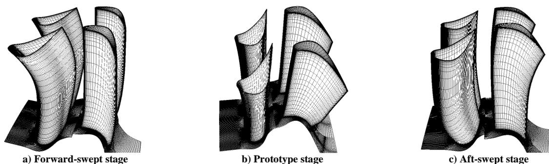
Figure 1. Three-dimension blade
