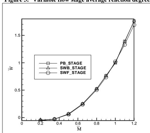
Figure 5. Variable flow stage average output power
