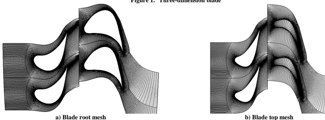
Figure 2. Mesh schematic diagram of blade root and top
