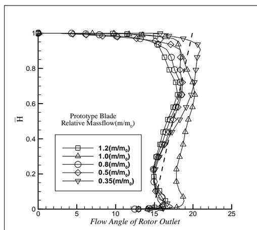
c) Forward-swept rotor cascade outlet flow angle
