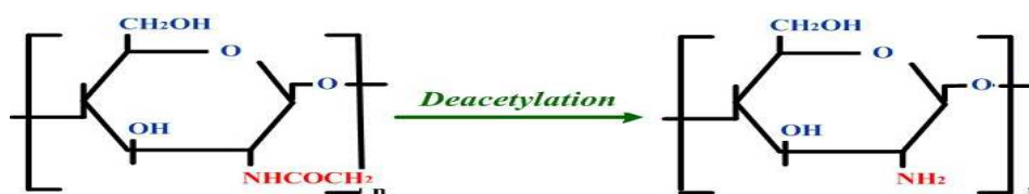
Figure 1: Molecular structures of chitin and Chitosan
