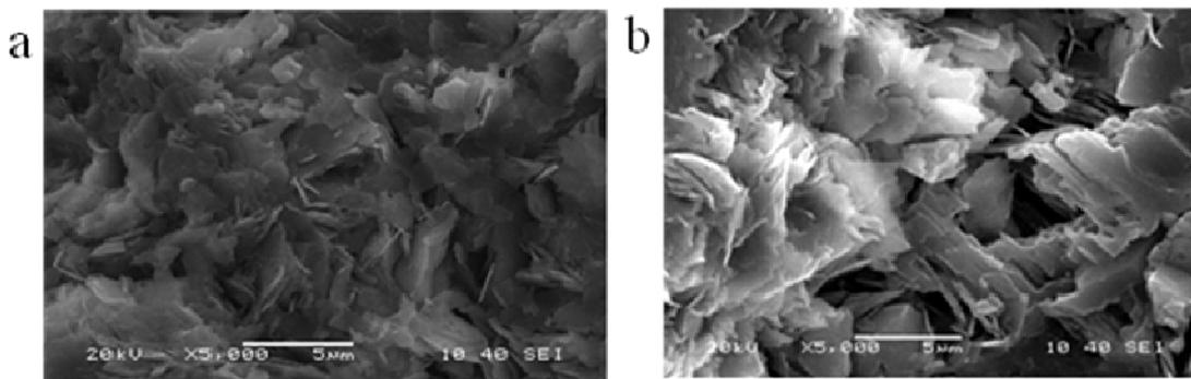
Figure 1. SEM images of modified zeolite (a)Natural zeolite, (b)Modified zeolite
