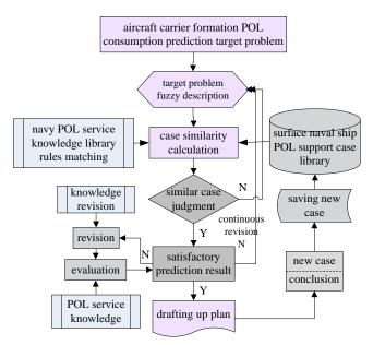
Fig.1 Process for adaptive case reasoning based aircraft carrier formation POL consumption prediction
