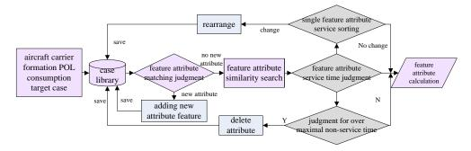
Fig.7 Aircraft carrier POL consumption case feature attribute optimizing process
