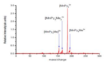
Figure 3. Mass spectrum of manganese pyridine dication complex ion when methane gas was introduced
