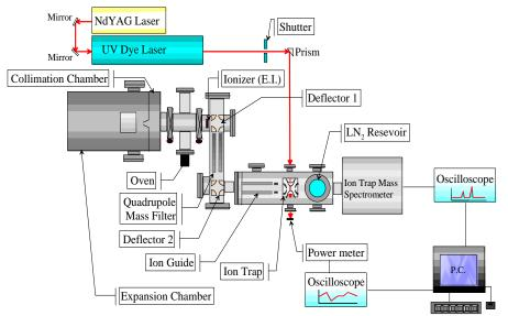
Figure 1. The diagram illustrating the experimental set up
