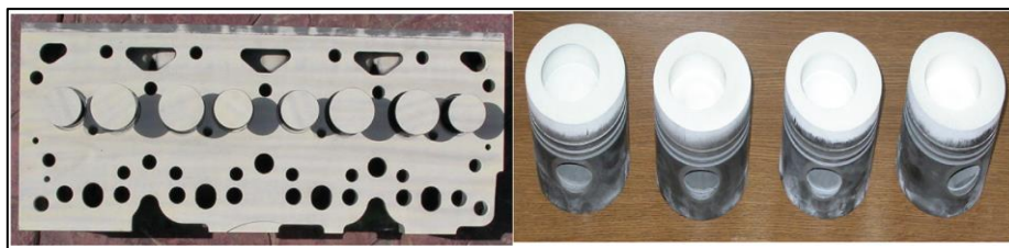
Figure 2: The Ceramic-Coated parts of the test engine
