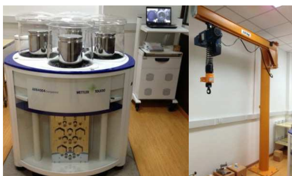
Fig. 1: AX64004 comparator installed in NIM and crane used for lifting weight
