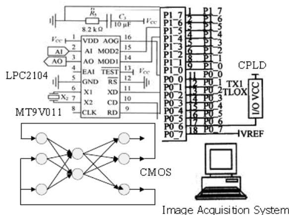
Fig. 2. CMOS Image Sensor to Design Image Acquisition System
