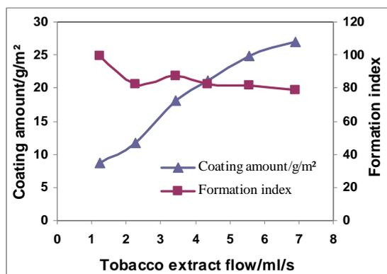
Fig. 2. Coating amount and sheet formation as a function of tobacco extract flow (\*coating speed was 20m/min, solid content of tobacco extract was 41.2%)
