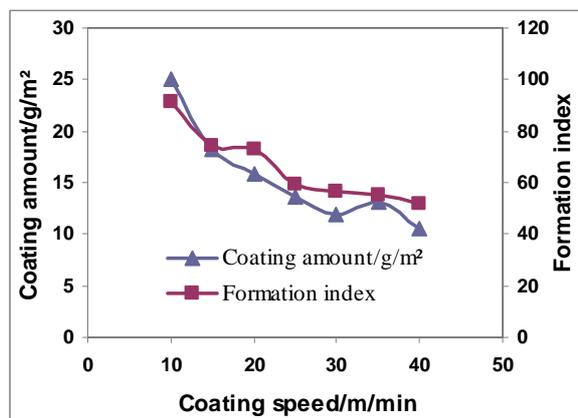
Fig. 3. Coating amount and paper sheet formation as a function of coating speed (\*solid content of the tobacco extract was 41.2%, tobacco extract flow was 3.45ml/s)
