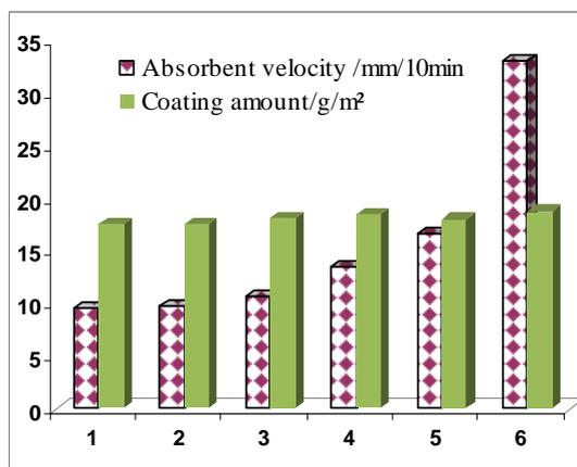
**Fig. 5. Coating amount as a function of absorbent velocity of reconstituted tobacco sheets (\*solid content of the tobacco extract was 41.2%, temperature was 22 ° C, coating machine speed was 10m/min, tobacco extract flow was 4.35 ml/s)**
