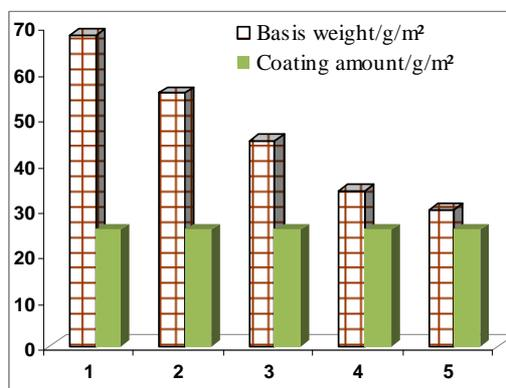
Fig. 4. Coating amount as a function of basis weight of reconstituted tobacco sheets(\*solid content of the tobacco extract was 41.2%, temperature was 22 °C, coating machine speed was 10m/min, tobacco extract flow was 4.35 ml/s)
