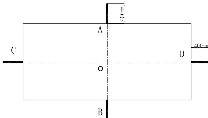
**Fig.7 Roadway surface displacement monitoring sections arranged**
