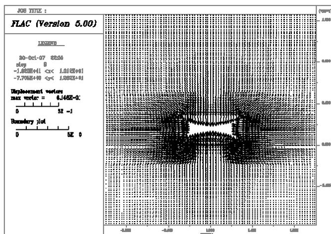
**(a)** Vector displacement of the anchor net support
