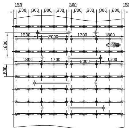
**Fig.2 Anchor beam support program**
