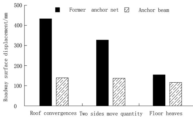
Fig.5 Surface displacement of the roadway
