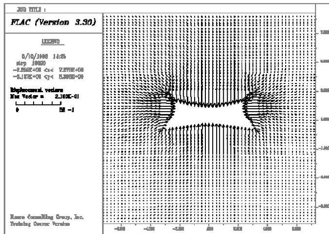
(b) Vector displacement of the anchor beam support
