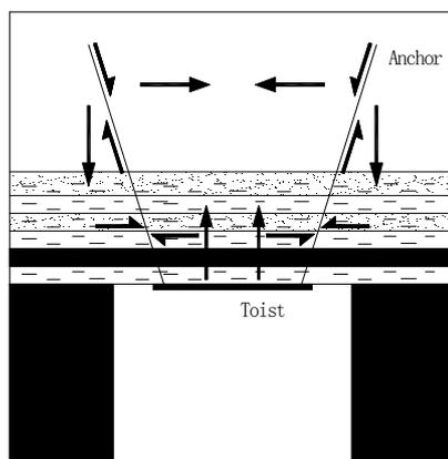
Fig.1 Large section compound roof anchor beam supporting Schematic
