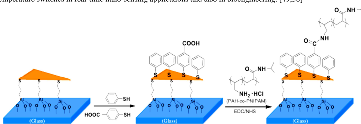
Figure 17: Schematic representation of the design of thermoresponsive polymer-functionalized plasmonic nanosensor
