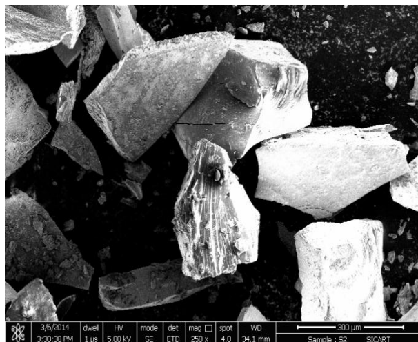
Figure: 6 SEM of borax cross-linked CMGG
