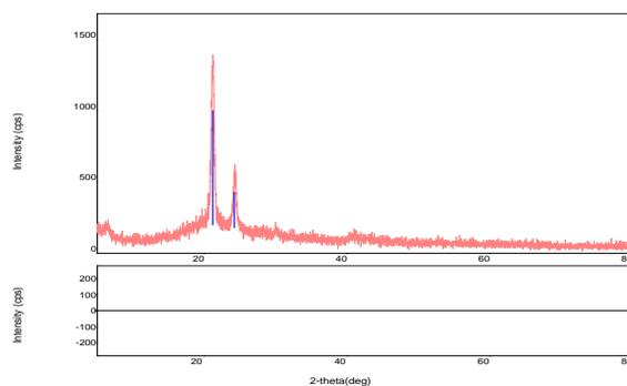
**Figure 5. X-Ray Diffractogram of PDDS**
