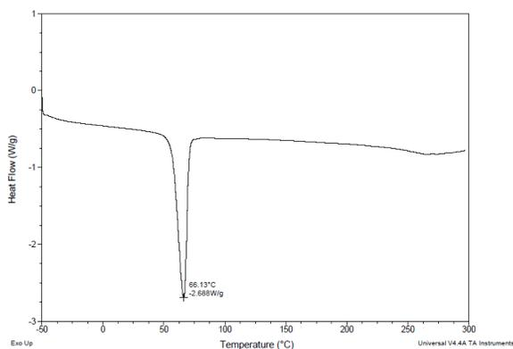
**Figure 4. DSC Thermogram of PDDS**
