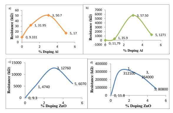
Figure 4. Resistance thin layer of ITO-Al a) 4 times coating, b) ITO-Al 5 times, and thin layer of ITO-ZnO c) 4 times coating and d) 5 timess coating
