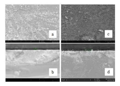
Figure 3. SEM images of the surface of the ITO-ZnO 5% thin film after being calcinated at 500°C with magnification (a) 5000 times, (b) 2000 times and surface of the ITO-Al 5% thin film after calcinating at a temperature of 550°C (c) 5000 times, (d) 2000 times magnification
