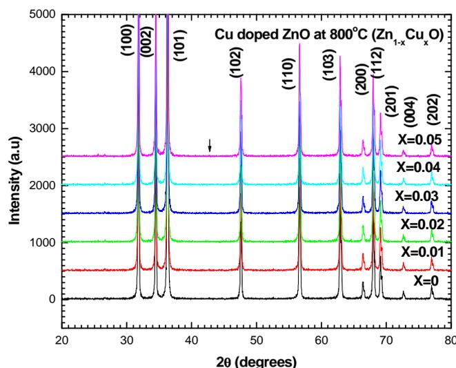
**Fig. 1 XRD patterns of pure ZnO and Zn<sub>1-x</sub>Cu<sub>x</sub>O nanoparticles at 800°C**
