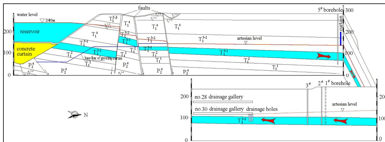
Fig. 2: Distribution of stratas, faults, confined water table and leakage pathway around Xiaolangdi left dam
