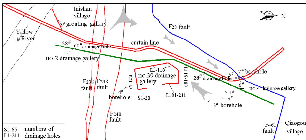
Fig. 1: Distribution of faults, no.30 drainage gallery, and observation boreholes at left abutment of Xiaolangdi Hydropower Station
