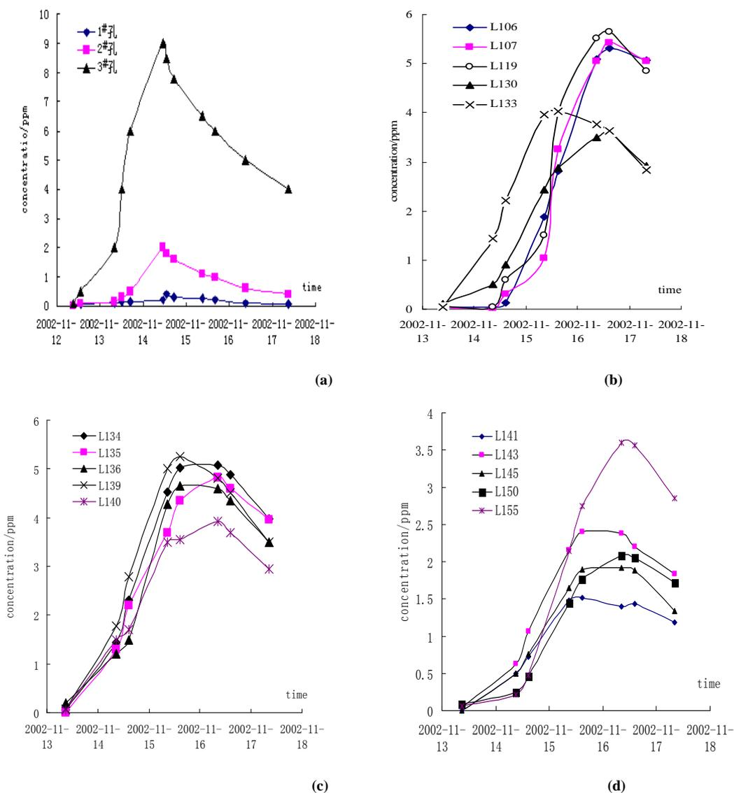
Fig. 4: Injected tracer detected in 1<sup>#</sup>-3<sup>#</sup> boreholes and part drainage holes in no.30 drainage gallery
