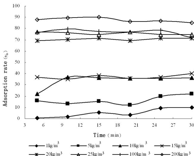
Fig.3 Adsorption rate of arsenic by coarse sediment in different time
