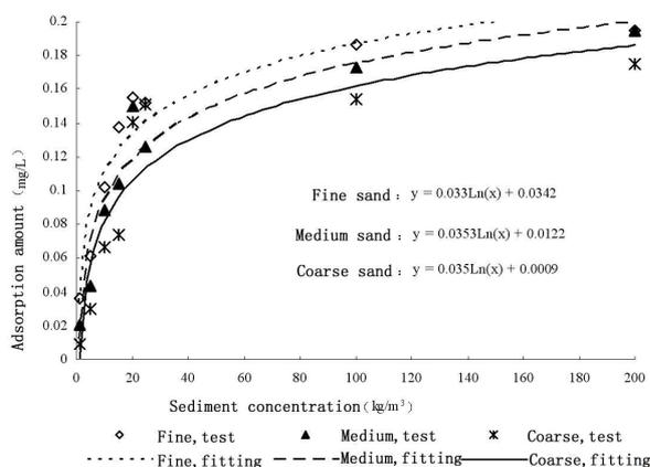
Fig.4 Adsorption curve of arsenic by measured and fitting
