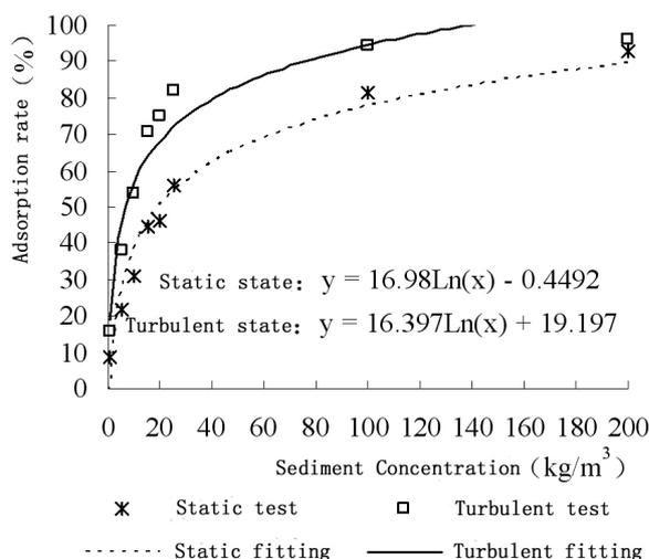
Fig.5 adsorption rate of arsenic in the hydrostatic and dynamic conditions
