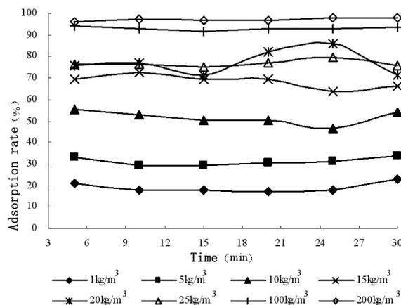
Fig.1 Adsorption rate of arsenic by fine sediment in different time
