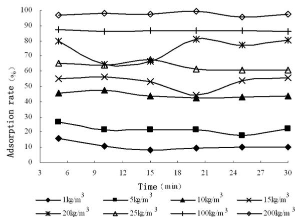
Fig.2 Adsorption rate of arsenic by medium granular sediment in different time
