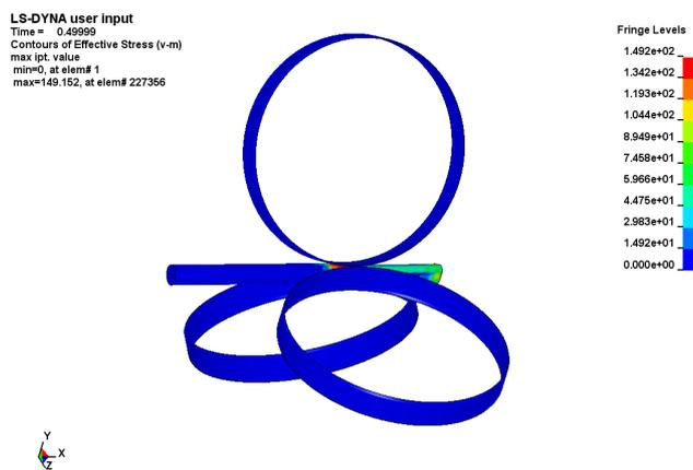
Fig. 3: Stress diagram of rolling bitten into the first pass stress
