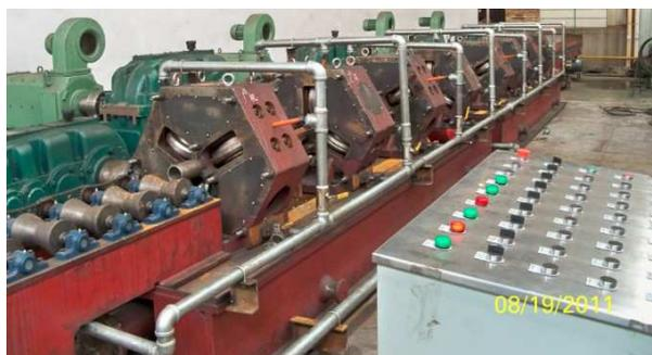
Fig. 1: Y-shaped three-roll mill production line
