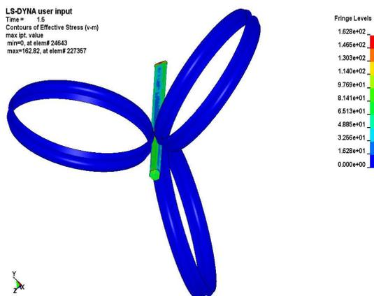
Fig. 5: Stress diagram of rolling bitten into the second pass stress
