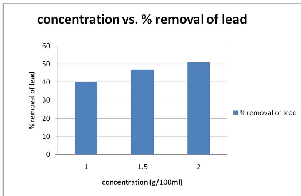
Fig 4: Concentration vs. adsorption of lead using the inner skin of cassava
