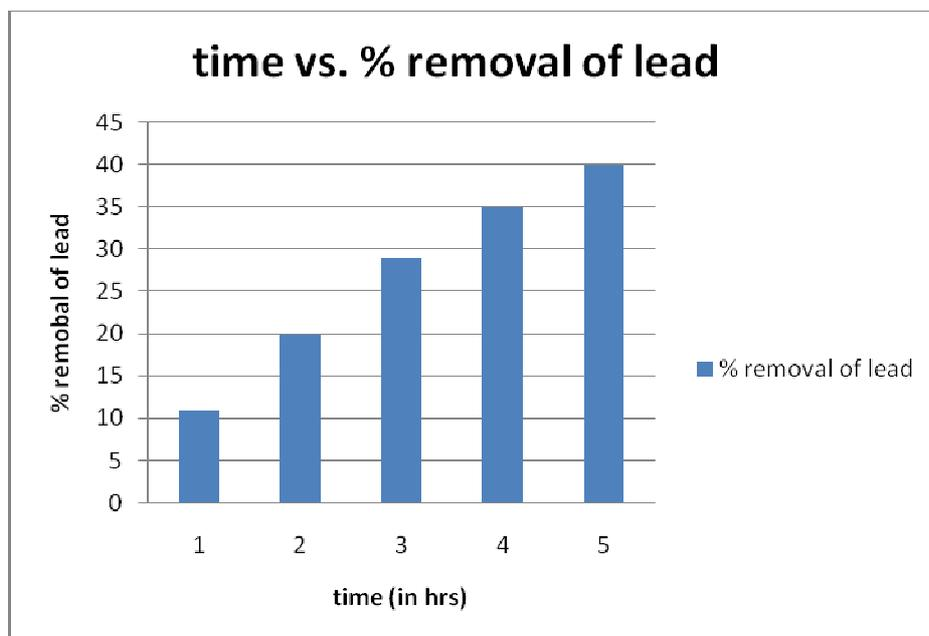
Fig 2: Time vs. % removal of lead using the inner skin of cassava
