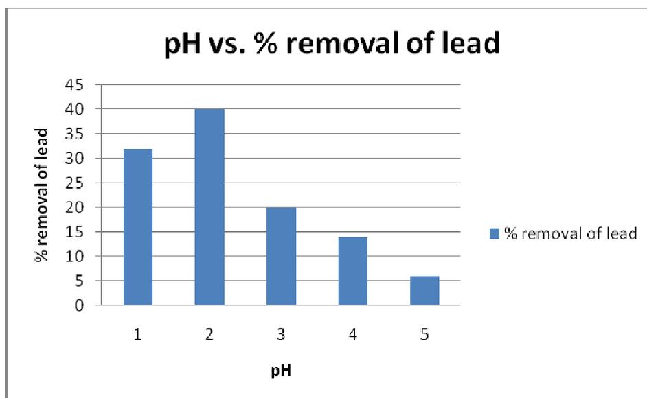
Fig 1: pH vs. adsorption of lead using the inner skin of cassava
