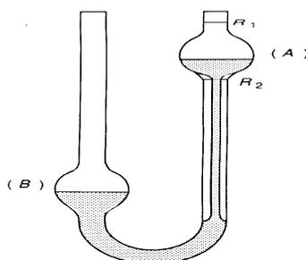
Figure 2 :Ostwald viscometer
