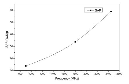
Figure 3: Variation in specific absorption rate with varying frequency
