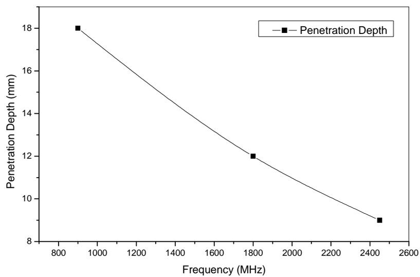
Figure 1: Variation in penetration depth with varying frequency
