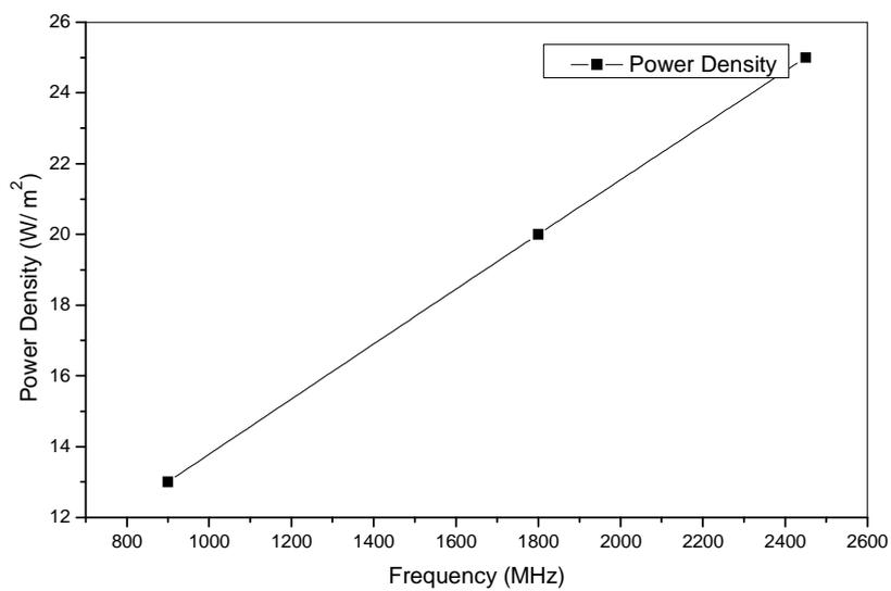
Figure 2: Variation in power density with varying frequency
