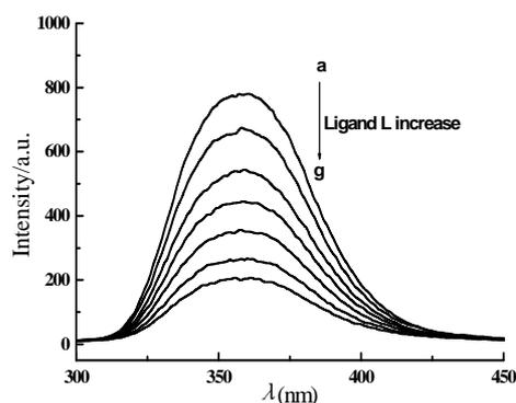
**Fig. 2** Fluorescence spectra of the complex with increasing amounts of the ligand at pH 7.0 and T = 25°C
