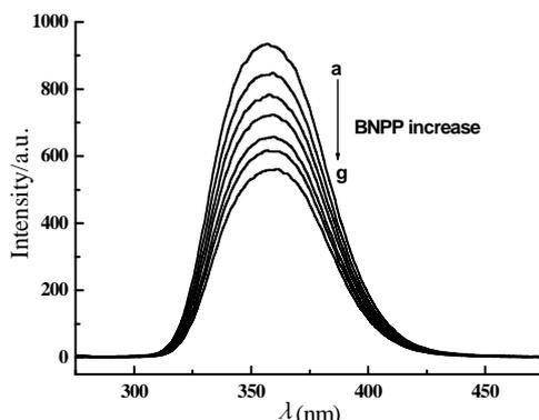
Fig. 4 Fluorescent spectra of the complex with increasing amounts of BNPP at pH 7.0 and T = 25°C.  $\lambda_{\text{ex}}=254 \text{ nm}$ ,  $[\text{complex}] = 5 \times 10^{-5} \text{ mol} \cdot \text{dm}^{-3}$ ,  $[\text{BNPP}] = 5.0 \times 10^{-3} \text{ mol} \cdot \text{dm}^{-3}$ , BNPP supplement 5  $\mu\text{L}$  per scan, a-g: 0-30  $\mu\text{L}$
