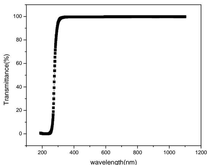
**Fig.4: Transmittance spectrum of cadmium sulphate hydrate crystal**
