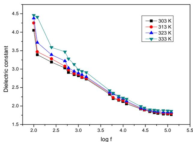
Fig.6: Variation of dielectric constant with frequency at different temperatures for CDSH crystal
