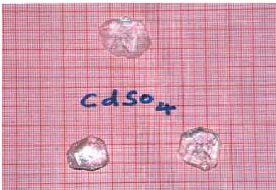
Fig.1: Grown crystals of cadmium sulfate
