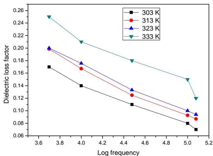
Fig.7: Variation of dielectric loss with frequency at different temperatures for CDSH crystal
