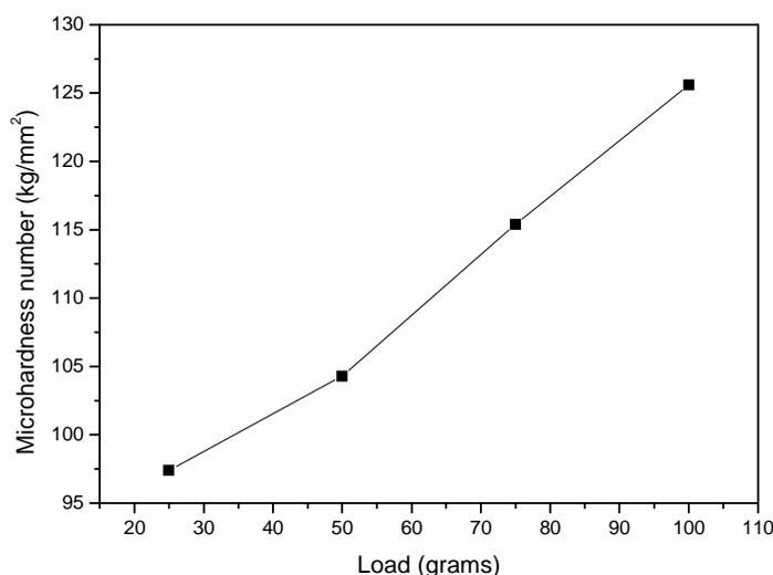
Fig.5: Plot of hardness number versus the applied load for cadmium sulfate crystal
