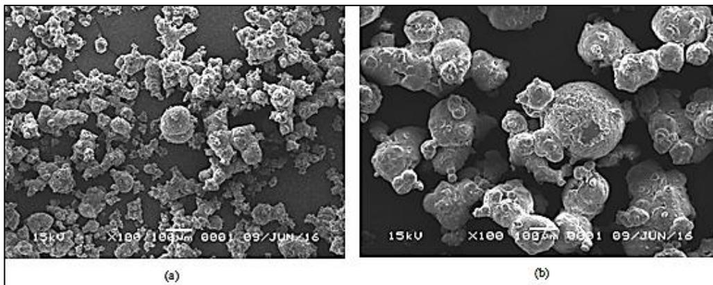
Figure 2: Scanning electron microscopy (a) placebo microcapsules and (b) urea microcapsules at 100x magnification, at 15 kV and 12 mA
