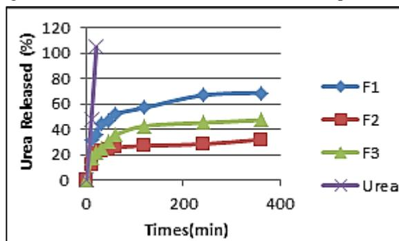
**Figure 4: Release profile of urea from microcapsules in distilled water medium**
