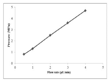
Figure 2. Permeability of the Methacrylate-based monolith column
