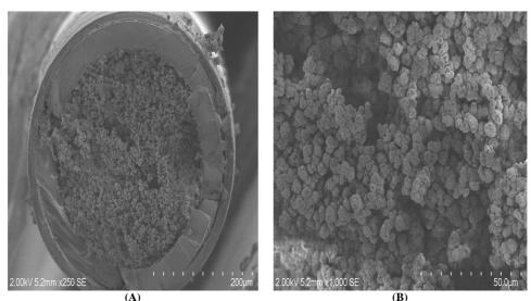
Figure 1. Scanning Electron Microsphotograph of monolith column (A) 250x (B) 1000x
