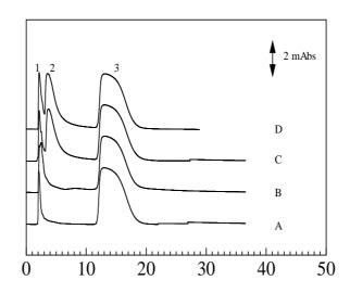
Figure 5. Chromatogram of inorganic anions in biomaterial samples. (1) IO<sub>3</sub><sup>-</sup>, (2) BrO<sub>3</sub><sup>-</sup>, (3) NO<sub>2</sub><sup>-</sup>. Column: 100 mm x 0.32 mm i.d. Flow rate 4 μL/min. Wavelength of UV detection 210 nm. (A) *Sapodilla*, (B) *Malay apple*, (C) *Lima bean*, (D) *Arenga pinnata*
