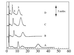
Figure 3. Effect of different kind of mobile phase on the separation of anion. (1)  $IO_{3^-}$ , (2)  $BrO_{3^-}$ , (3)  $NO_{2^-}$ , (4)  $Br^-$ , (5)  $NO_{3^-}$ ; Column 100 mm x 0.32 mm i.d.; Flow rate 4 µL/min. Mobile phase (A) NaCl (B) LiCl (C) KCl (D) NH<sub>4</sub>Cl (E) RbCl
