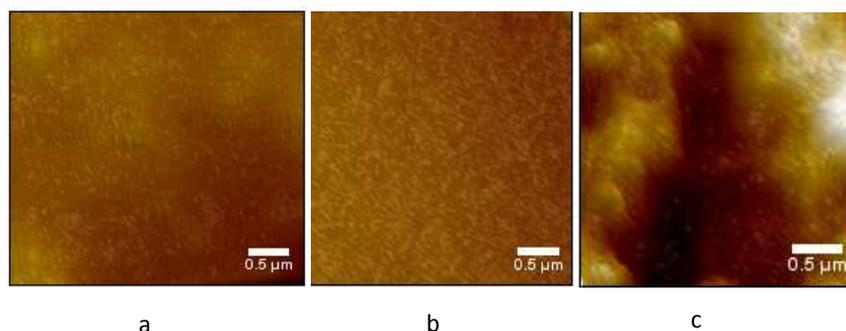
**Fig.2. Atomic Force Microscopy Image of (a) Xylan control film (0% CNW); (b) Xylan film reinforced with 2% CNW; (c) Xylan film reinforced with 10% CNW**
