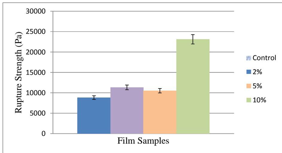
**Fig.3. Rupture Strength of Xylan Nanocomposite Films Reinforced with Different Levels of Bamboo Cellulosic Nanowhiskers (CNW)**
