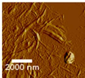
**Fig.1. Atomic Force Microscopy Image of Bamboo Cellulosic Nanowhiskers**
