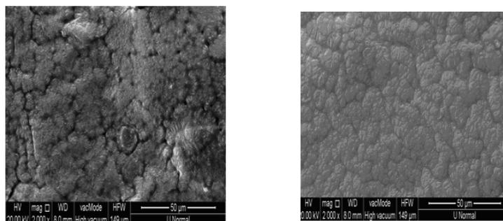
**Figure 6** SEM images of collagen composite films: (a) with crosslinking agent, (b) without crosslinking agent
