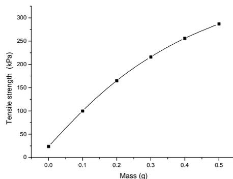
Figure 2 Effect of the amount of sodium alginate on the tensile strength of collagen films
