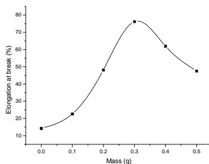
Figure 3 Effect of the amount of sodium alginate on the elongation at break of collagen films
