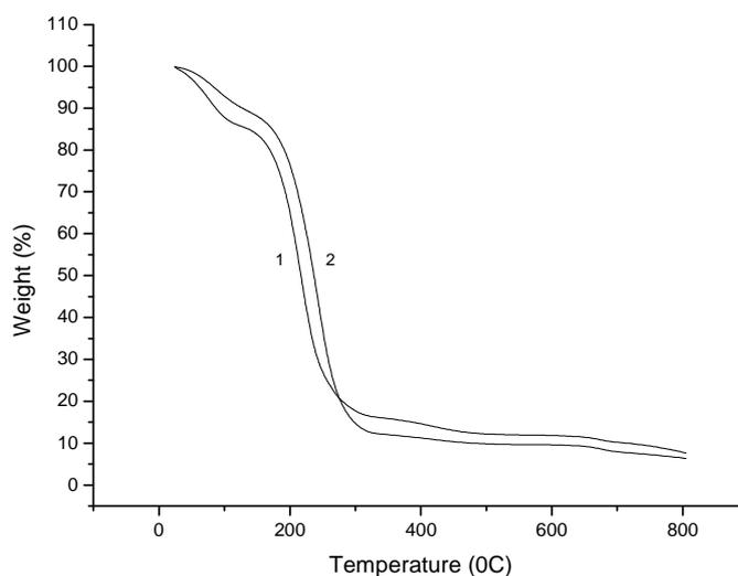
Figure 4 TGA curves of collagen films: 1 – with addition of sodium alginate; 2 – without addition of sodium alginate
