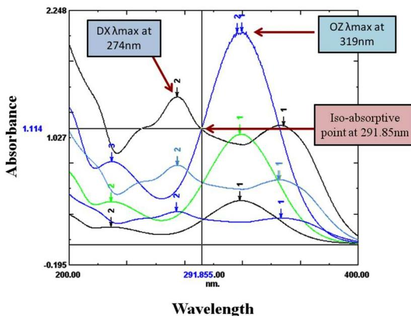
Figure 4: Overlay spectra of ornidazole (OZ) and doxycycline (DX) illustrating  $\lambda_{\max}$  of both the drugs and their iso-absorptive point
