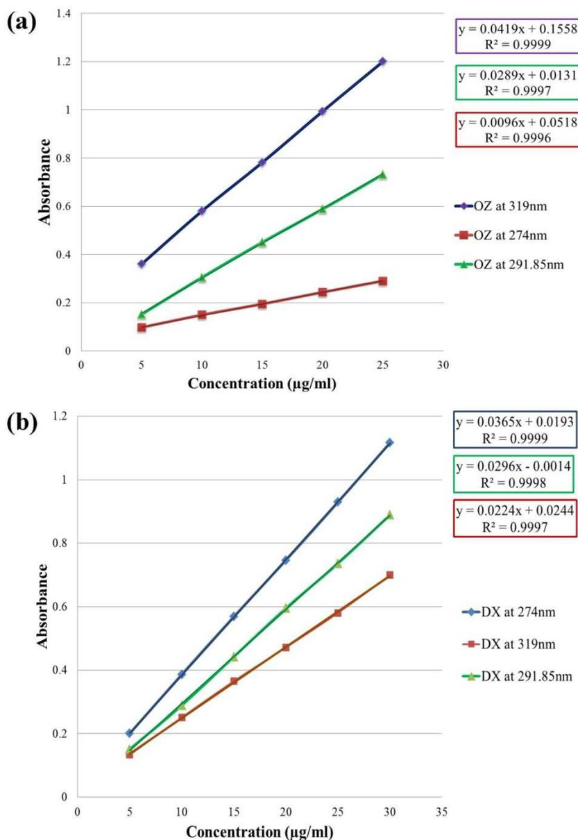
Figure 7: Calibration curve of a) OZ and b) DX at 319, 274 and 291.85 nm
