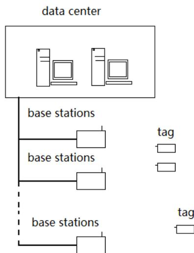
Figure 1 Overview of the Personnel Positioning System Based on RFID
