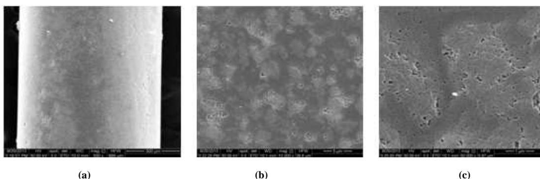
**Fig. 1** Scanning electron micrographs of polymer monolithic rod. (a) 300×, (b) 10000×, (c) 50000×
