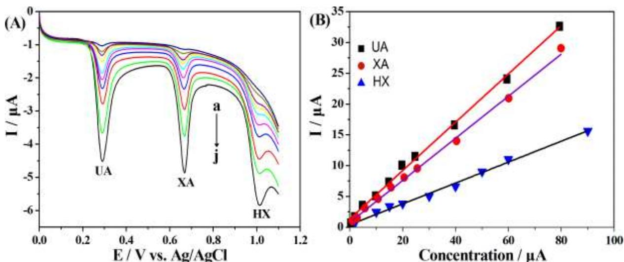
Fig. 6 (A) LSV of different concentrations of UA, XA (a-j: 0.2, 2, 5, 10, 15, 20, 25, 40, 60, 80  $\mu\text{M}$ ) and HX (a-j: 0.5, 2, 10, 15, 20, 30, 40, 50, 60, 90  $\mu\text{M}$ ) on PCA/GCE in pH 6.5 PBS. (B) Concentration calibration curve of the LSV current response for UA, XA and HX
