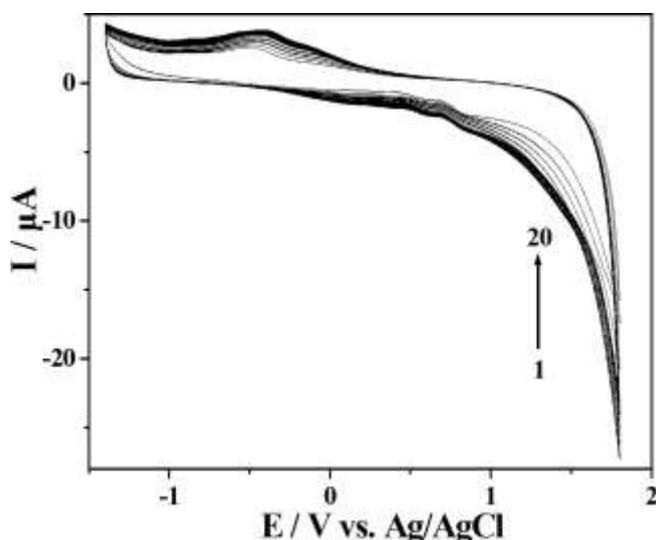
Fig. 1 CV of CA in electropolymerization process from 1 to 20 cycles. CA:  $2.5 \times 10^{-3}$  M; supporting electrolyte: pH 7.4 PBS containing 0.01 M  $\text{KNO}_3$ ; scan rate:  $100 \text{ mV s}^{-1}$
