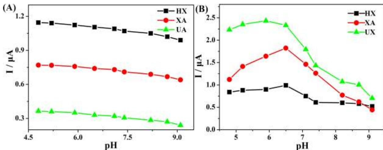
Fig. 4 Effects of pH on the anodic peak potential (A) and anodic peak current (B) of 50  $\mu\text{M}$  UA, XA and HX on PCA/GCE. Scan rate: 50  $\text{mV s}^{-1}$
