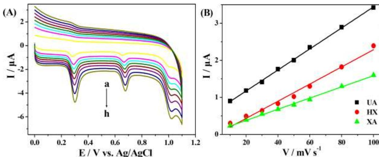
Fig. 3 (A) CVs of 50  $\mu\text{M}$  UA, 25  $\mu\text{M}$  XA and 50  $\mu\text{M}$  HX mixture solution on PCA/GCE at with different scan rates (a-h: 10, 20, 30, 40, 50, 60, 80, 100  $\text{mV s}^{-1}$ ) in pH 6.5 PBS. (B) Plots of the oxidation peak current versus the scan rate
