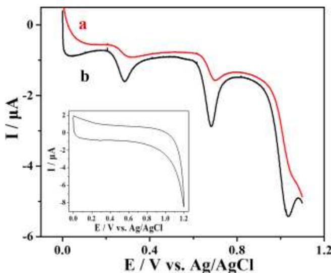
Fig. 2 LSVs of bare GCE (a), PCA/GCE (b), in pH 6.5 PBS containing  $20 \mu\text{M}$  UA,  $40 \mu\text{M}$  XA and  $80 \mu\text{M}$  HX with a scan rate of  $50 \text{ mV s}^{-1}$ . Inset: CV of PCA/GCE in pH 6.5 PBS
