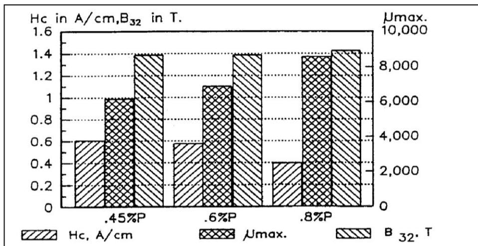
Figure 3: Effect of phosphorus content in Fe-5%Sn-P alloys, samples compacted at 589 MPa, sintered for 30 minutes at 1250°C in H<sub>2</sub> atm
