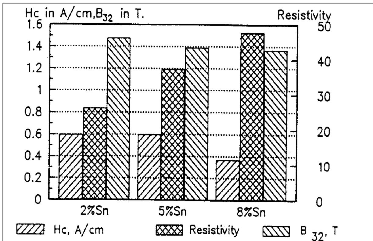
Figure 2: Effect of tin content in Fe-Sn-0.45%P alloys, samples compacted at 589 MPa, sintered for 30 minutes at 1250°C in H<sub>2</sub> atm
