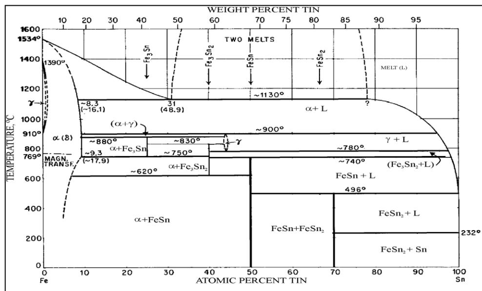
Figure 1: Phase diagram of Iron-Tin alloys [5]
