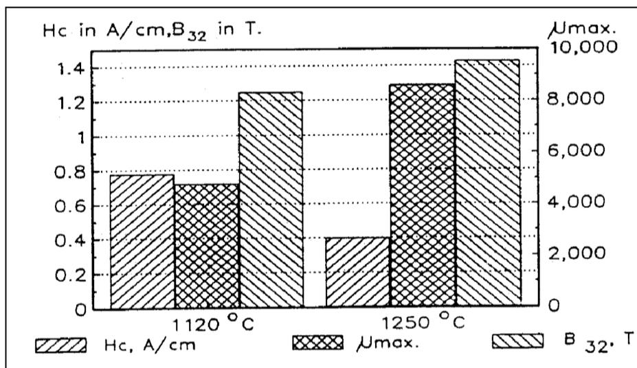
Figure 4: Effect of sintering temperature on Fe-5%Sn-0.8%P alloy, samples compacted at 589 MPa, sintered for 30 minutes at 1250°C in H<sub>2</sub> atm
