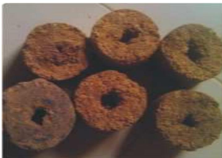
**Plate 2: Bambaranut shell briquettes produced**
