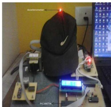
Fig 11 Accelerometer Interface to PC Kit
