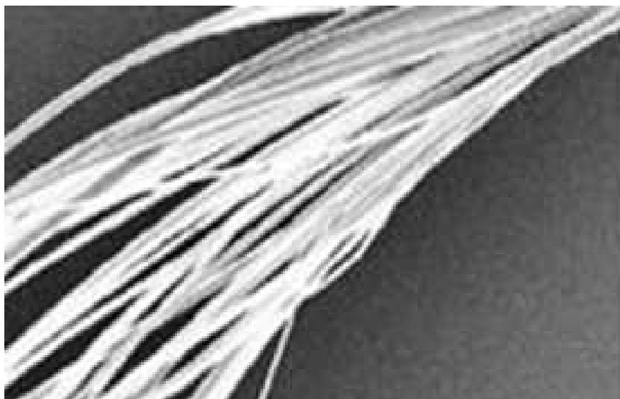
Fig. 7: SEM of poly (L- lactic acid) fibers using phase separation method
