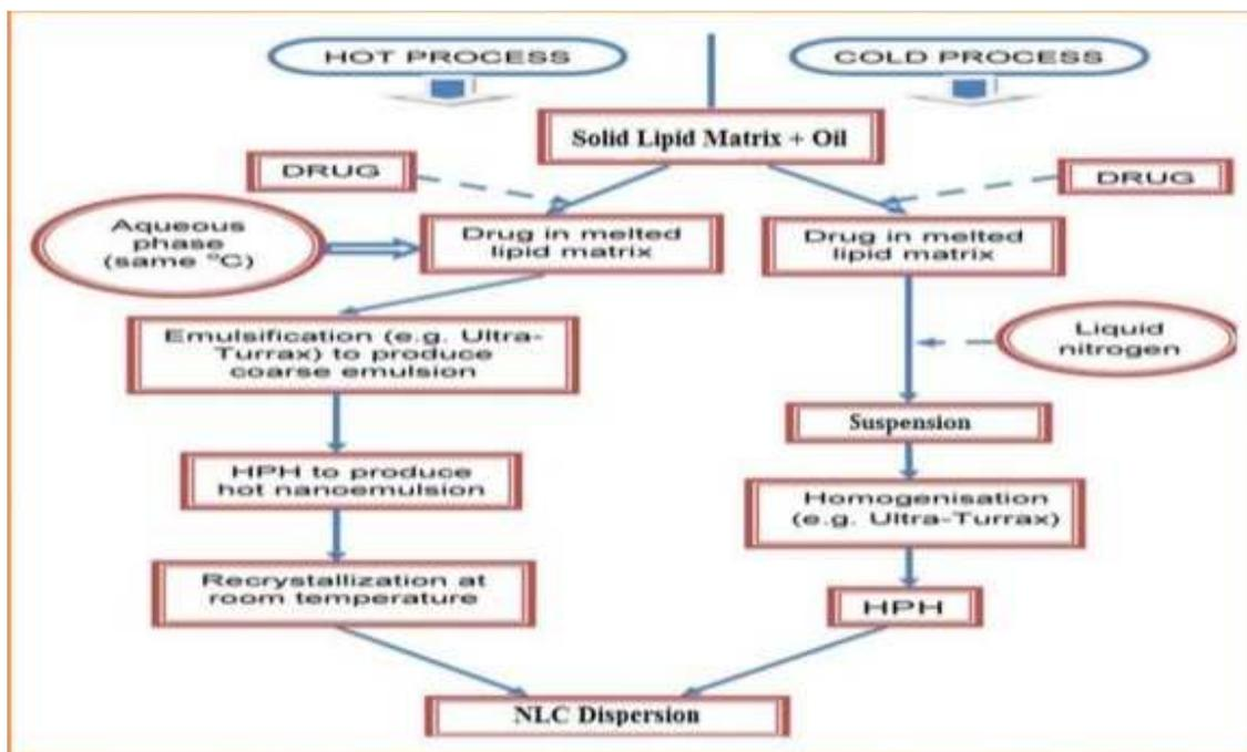
FIG.6 Flow chart of Hot HPH and Cold HPH
