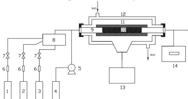
**Fig. 1: Schematic diagram of microwave catalytic reactor**
