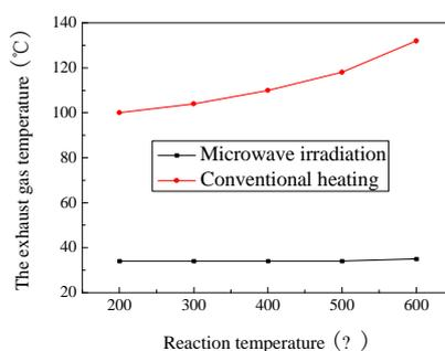
**Fig.2** The comparison of exhaust gas temperatures under different reactor systems (Reaction conditions: molar fraction of O<sub>2</sub>, 5.88%; molar fractions of NO, 1×10<sup>-3</sup> and GHSV, 1920 h<sup>-1</sup> and ambient temperature, 32°C)
